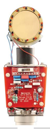
Frequency Range: 20Hz-20Khz Sensitivity: 12 mV/Pa Impedance: 200 ohms
