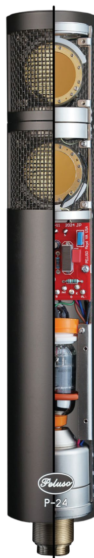
The upper capsule of the P-24 can be roated in 15-degree increments up to 180 degrees, relative to the fixed, bottom capsule.
